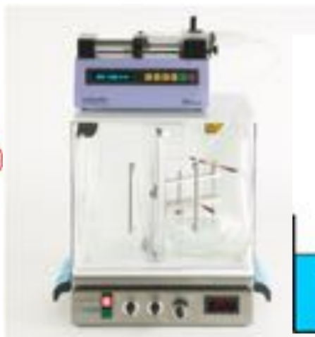
Var V1 (Nisco, CH) - electrostatic capsule generator
